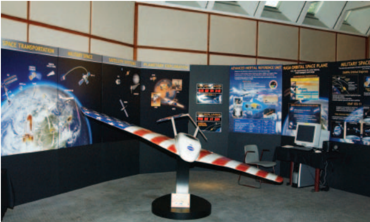
Draper Laboratory, Langley Research Center, and the Jet Propulsion Laboratory are combining their talents to collaborate on future programs, particularly those directed at the exploration of Mars. Pictured above is the ARES rocket-powered Mars airplane, which is part of a proposed Mars Scout mission designed to perform an aerial regional-scale environmental survey of Mars.
