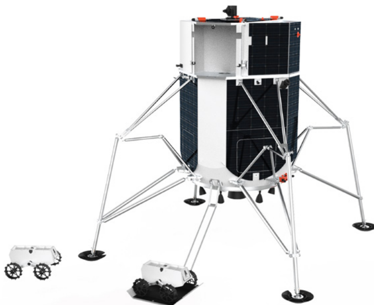
Figure 2 – Artemis-7 Lander Payload accommodations and volume
