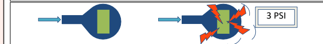
Figure 3: Preliminary testing was conducted using balloons and tape resulting in burst pressure values above 3 psi.
