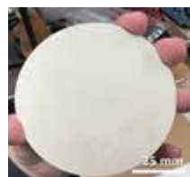
Figure 2. Sintered slip cast Si 3 N 4 sample.
