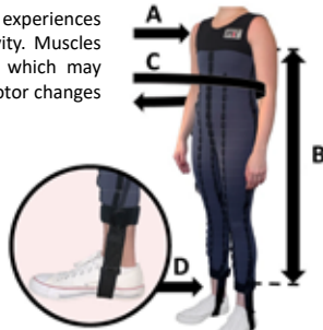
Fig. 1. The Mk-7 Gravity Loading Countermeasure Skinsuit with A) shoulder yoke, B) longitudinal fabric tension in the loading material, C) circumferential fabric tension in the loading material, and D) stirrups secured under the sole of shoes with rigid insoles. (modified from [5]).
