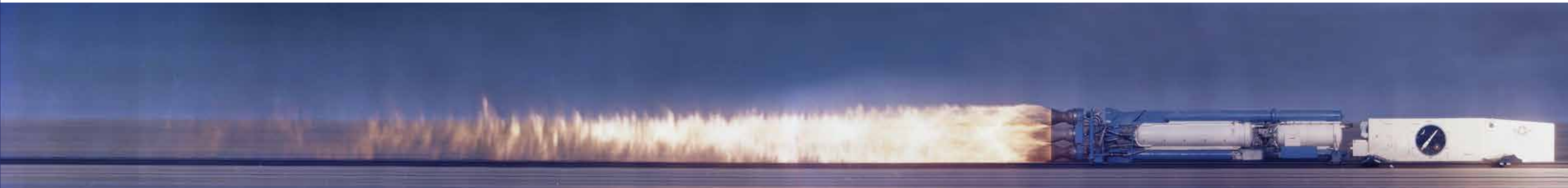
Rocket sled test of MPMS/AIRS (circa 1980)
