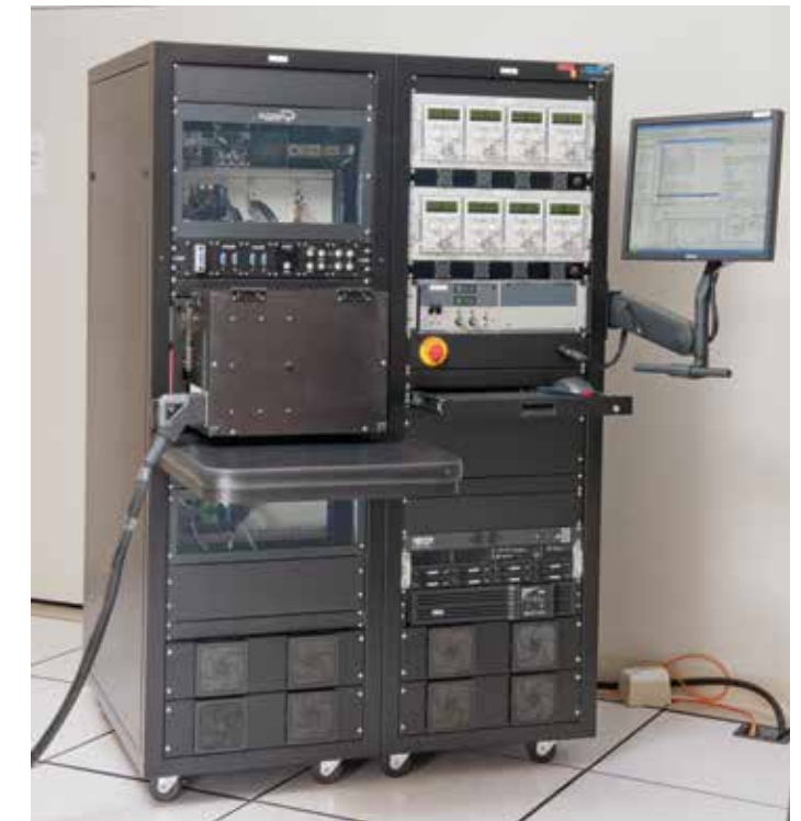
The UTS developed by Draper provides a modular approach for testing both existing and new inertial instruments.
