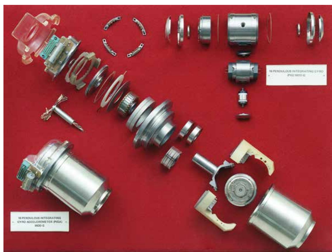
The 16 PIGA Mod G was used on Minuteman III, which was deployed in 1970.
