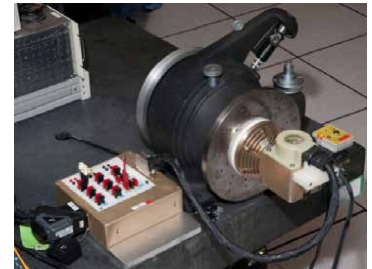
The UTS dividing head used for mounting the sensor for testing
