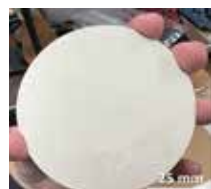
Figure 2. Sintered slip cast Si 3 N 4 sample.
